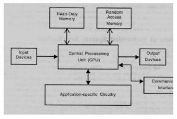
Now, let us see the details of the various building blocks of the hardware of an embedded system. As shown in Fig. the building blocks are;
